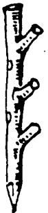
Temp Stick: Used for heat control. The lower the fork, the hotter. Pegs in the stick work too.
